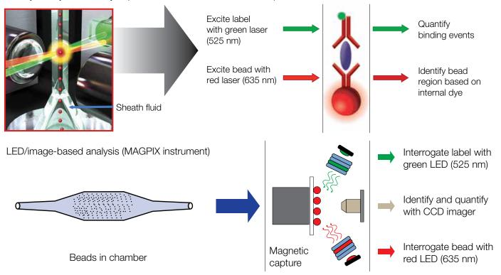
Figure 2. Luminex xMAP technology uses either light-emitting diodes (LEDs) or lasers to measure the levels of several (typically 5 to 30) targets in a single sample.
